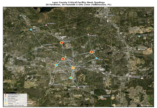
Fig. 3. Simulated Resilience Node deployment over Leon County, Florida: 20 real critical facilities (hospitals, EOC, fire stations, schools/shelters, universities) joined by the 39 feasible 5 GHz mesh links. Ringed markers are gateway-capable (satellite-backhaul) sites. Imagery: Esri World Imagery.
